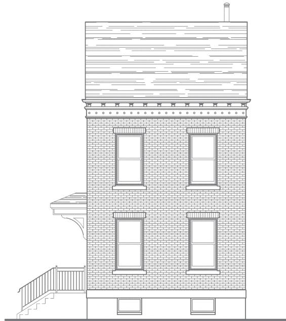
Building Elevation with Brick Soldier Course Header
